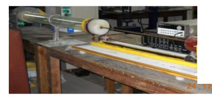
Fig.1 Standing wave apparatus
