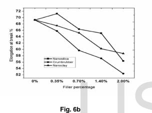
Effect of fillers on tensile strength (6a) and elongation at break (6b)
