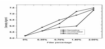
Fig. 3 Effect of fillers on density
