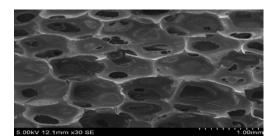
Fig. 4b 1.4%Nano silica in PU foam
